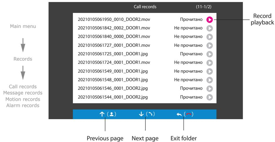
Press ▶ icon on the right side of the file name to start current file playback. Also you can stop playback, delete current file, set up volume or get back to the list of video files using the buttons on the bottom of the screen:
