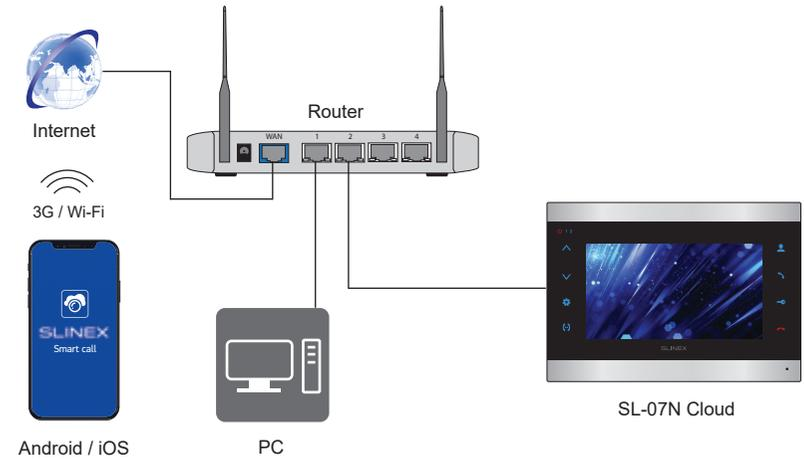
Diagram 2. SL-07N Cloud wireless Wi-Fi network connection.
